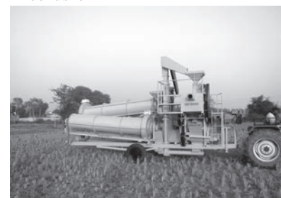
Fig. 2 RHS view of tractor operated paddy thresher-cum-dryer-cum-dehusker
