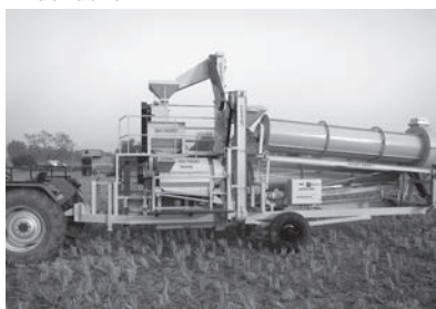
Fig. 1 LHS view of tractor operated paddy thresher-cum-dryer-cum-dehusker
