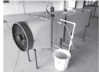
Fig. 5 Fabricated TSEC system with set up
