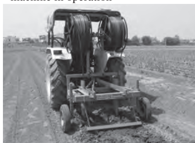
Fig. 4 A view of subsurface drip laying machine in operation
