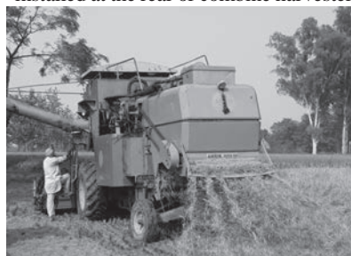
Fig. 4 Operational view of Super SMS installed at the rear of combine harvester
