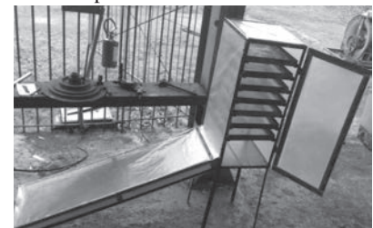
Fig. 1 Solar dryer of aromatic plants developed in research
