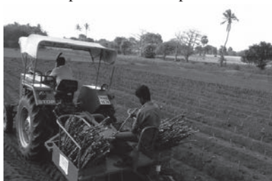
Fig. 7 Operational view of tractor operated cassava planter
