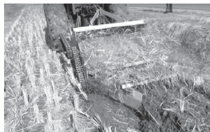
Fig. 5 Working view of tractor operated bund former machine
