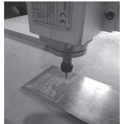
Fig. 15 Manufacture of PCB in 3-axis CNC Router
