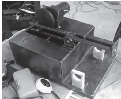
Fig. 4 Movement of connecting rod-crank mechanism, lower maximum position
