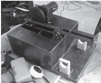
Fig. 3 Movement of connecting rod-crank mechanism, upper maximum position
