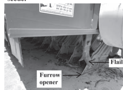
Fig. 2 Furrow opener and flail of happy seeder
