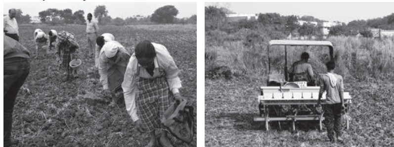
Fig. 5 Sowing of chickpea 2 seeds per hill by manual labor and by developed machine
