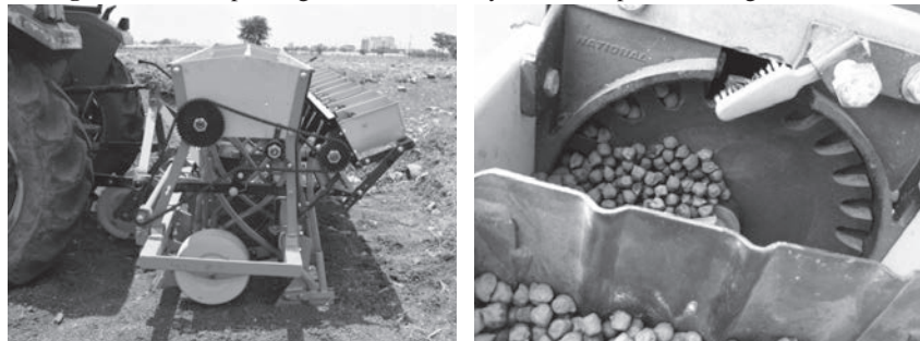
Fig. 3 Two seeds picking from seed box by the developed metering mechanism
