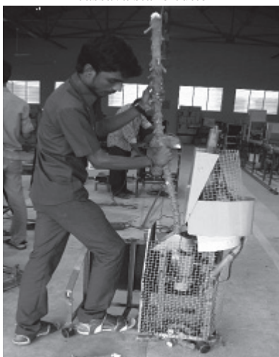
Fig. 3 Operational view of experimental cassava stake cutter
