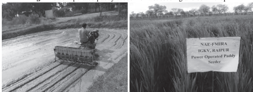
Fig. 7 Power operated paddy seeder for wet seeding and sown crop
