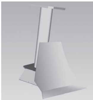
Fig. 2 Computer aided drawing of truncated mould board
