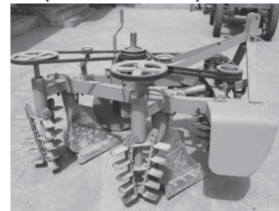
Fig. 8 A stationary view of tractor operated biomass incorporator
