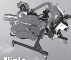
Niplo Levee Plastering Machine
