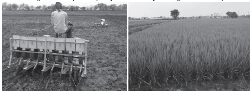
Fig. 6 Power operated paddy seeder for dry seeding and sown crop
