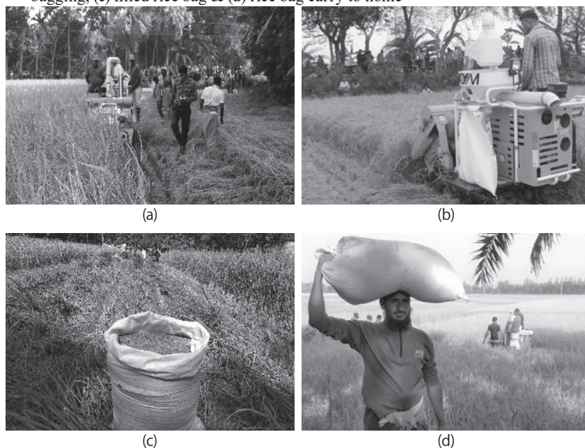
Fig. 3 Mechanical harvesting (a) harvesting by mini-combine, (b) harvesting and bagging, (c) filled rice bag & (d) rice bag carry to home
