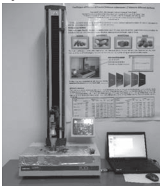
Fig. 2 Special testing device for pellet firmness
