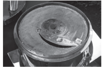
Fig. 4 View of the wooden cutting disc and the blade with a curved cutting front at the initial stage
