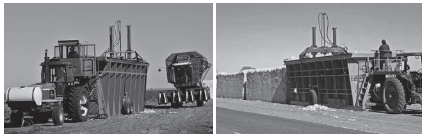
Fig. 7 A view of module builder in field during operation
