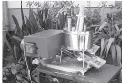
Fig. 3 Motorized manioc slicer with a gear reduction developed at the initial stage
