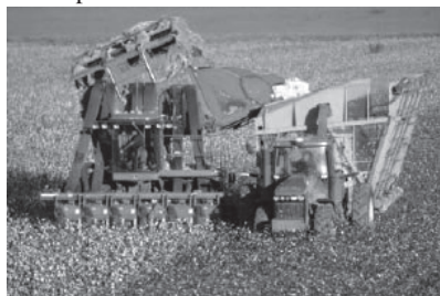
Fig. 6 Conventional basket picker stops on the row and unloads
