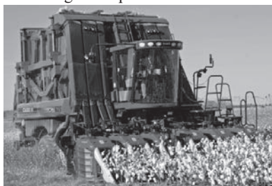
Fig. 4 A spindle type cotton picker during field operation
