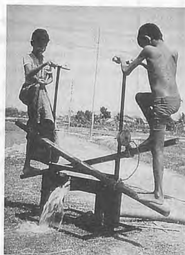
Fig.3 Bari Pump in Operation.
