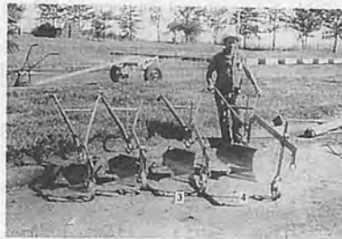
Fig. 4 Different sizes of reversible mouldboard plows Tamanduá/lapar. Numbers 3 and 4 are the last two at the right side of the figure.
