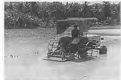
Fig. 2 Working of the rotavator at work in wet land.
