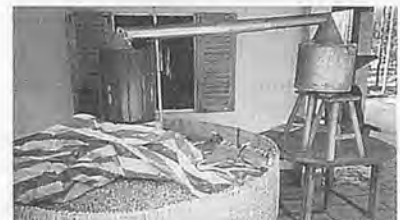
Fig. 3 Stove using pulverized and compressed coal as heat source for SRR-1 dryer, shown with peanut in the bin.
