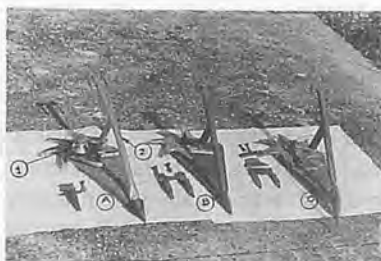
Fig. 6 Modified crop divider-starwheel and knife guard of cutterbar.
