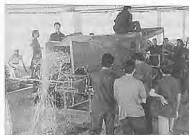
Fig. 7 Demonstrating the raspbar flow through thresher.
