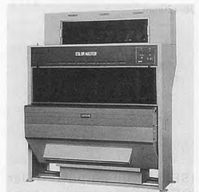
SATAKE Color Sorters with their quality optics and high-grade electronics allow the operator to make efficient separator on the basis of color. Model: GS40AG/AK/AP, GS60AG/AK/AP, GS80AG/AK/AP and CS500B. Major Application: Rice, wheat, coffee, corn, sunflower, beans, spices, etc.
