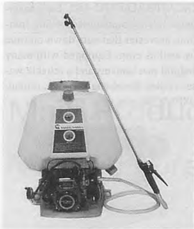
MARUYAMA Portable Power Sprayers MSO55D. Engine: Air-cooled, 2-cycle, output 22.6cc, Pump: Suction capacity 5.14/mm, max pressure 25 kg/cm 2 , Weight: 8.5 kg.
