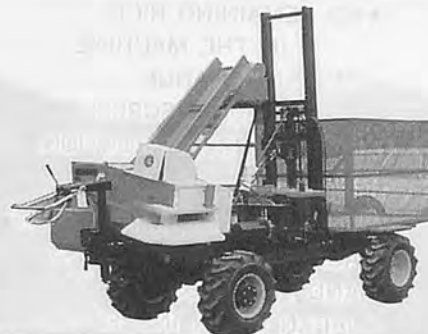
THE SMALL LEAF STRIPPING MACHINE (KC-2 MODEL)
