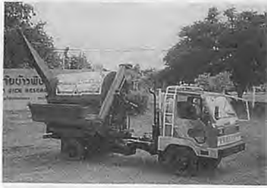
Fig. 4 Thailand has several manufacturers of truck-mounted threshers. There are a range of models made, for example, by Kaset Patana at their Pit-sanoluke factory, requiring 75 to 150 HP (56-90 kW). They can be equipped with a power feeder, tailings return, full grain cleaning system and conveyor to sacking chute. Capacity is around 3 t/h clean paddy for the 75 HP model, up to 7-12 t/h for the KPF-8 powered by a 150 HP engine. The largest model has an 0.5 m diameter rotor 2.3 m long (Photo provided by the Company).
