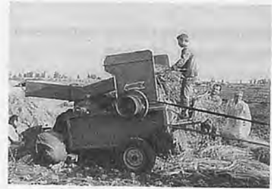
Fig. 10 Nile Delta farmers using an Egyptian-built dual-mode thresher for their paddy harvest. Capacity is around 1 t/h of rice and the drive power comes by belt from a tractor of typical size 65 HP. (Photo courtesy of Amir Khan).
