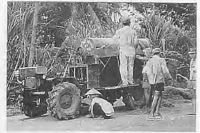
Fig. 5 Vietnam. This is a locally-built axial flow thresher being transported by canal barge to a field site on the Mekong Delta, South of Cantho (IRRI photo by Thomas Hargrove).
