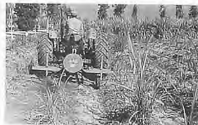
Fig. 5 Rotary weeder in action eradicating weeds in between the sugarcane plants.
