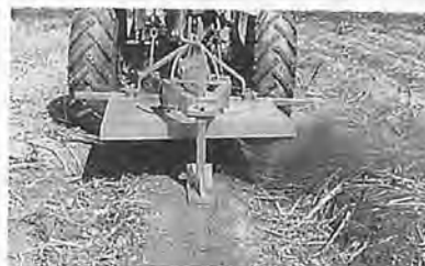
Fig. 7 Shaving of sugarcane stubbles with the stubble shaver.
