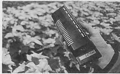
TELAIRE CO 2 Concentration Measuring Equipment 2001 VTC. Telaire 2001VTC can watch necessity of ventilation, control air stream, measure air speed and control ventilation with fan in greenhouse. It can measure temperature and CO 2 by the infrared NDIR technique and diagnose condition of greenhouse automatically. Measurement range: 0~3000 ppm, Display indicator: 4 figures, Battery usable hours before next recharging: 2,11 h (2 types).
