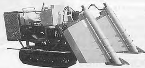
THE RIDING TYPE HARVESTER (TK-5...60PS)
