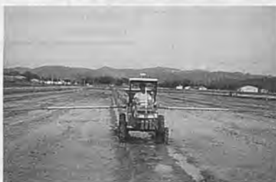
Fig. 4 Seeding by multi-purpose granule applicator.
