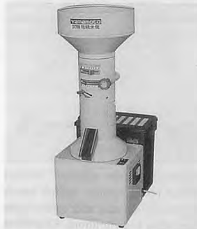
YAMAMOTO Rice Whitener Ricepal Series Model VP31T. High recovery rate. Immatured rice can be milled. No remaining rice in the machine. Easy-to-change milling screen. Durable construction. Milling system: vertical type single pass, Size (H × W × L): 850 × 330 × 450mm, Weight: 24kg, Power required: 0.3kW, Electric mains: single phase 100V (50/60Hz), Capacity: 30kg/h, Rpm: 1440/1730, Hopper holding capacity: 15kg, Safety device: Circuit protection.
