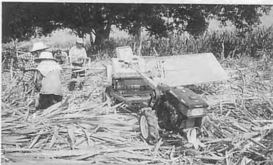
THE BABY LEAF STRIPPING MACHINE (MBC-250C)
