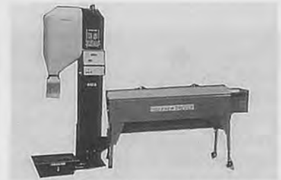
TIGER KAWASHIMA Rice Combi and Grader. Rice grading machine and automatic weighting and packaging.
