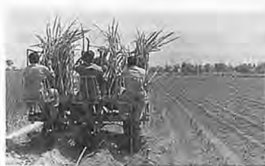
Fig. 8 Sugarcane planter at work in the field.
