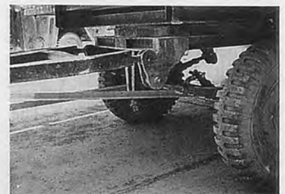
Fig. 6 Connecting the cross-arms to the trailer.
