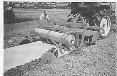
Fig. 6 Paper stretching operation using ordinary paper and mulching equipment.
