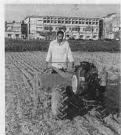
Fig. 2 Power tiller-operated groundnut planter cum-fertilizer drill in operation.
