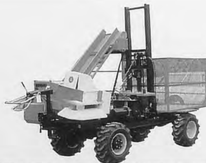
THE SMALL LEAF STRIPPING MACHINE (KC-2 MODEL)
