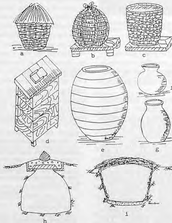
Fig. 2 Traditional storage structures commonly used in Orissa. (a) and (b) Straw storage structures, (c) Bamboo/reed storage structure, (d) Wooden storage structure (e), (f) and (g) Earthen storage structures, (h) and (i) Under-ground storage structures.
