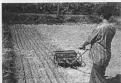
Fig. 2 Field operation of manually-operated paddy-cum-groundnut planter.
