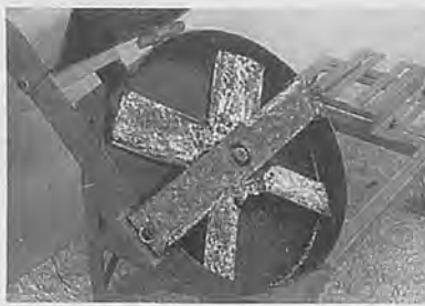
Fig. 1b The chopper blades: four rotating blades angled 10° upwards with respect to the counter-edge. The distance from the cutting plane to the floor of the housing is 25 mm, the theoretical length of chop.
