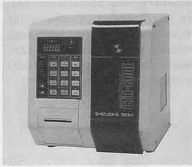
SHIZUOKA's Single Kernel Moisture Tester CTR-800E for rough rice, brown rice, wheat and barley.
