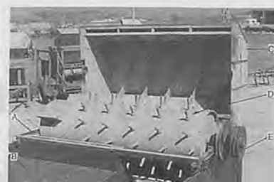
Fig. 2 Threshing unit. A) Concave, B) Feeding table, C) Drum cover, D) Threshing drum, E) Feeding mouth.
