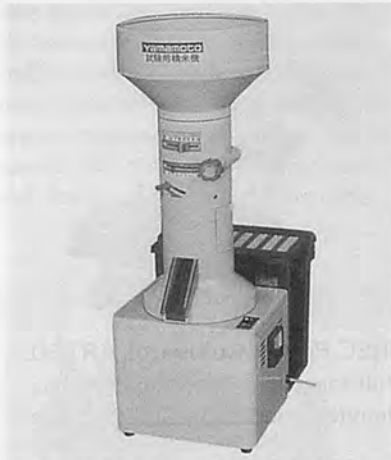
YAMAMOTO Rice Whitener Ricepal Series Model VP31T. High recovery rate. Immatured rice can be milled. No remaining rice in the machine. Easy-to-change milling screen. Durable construction. Milling system: vertical type single pass, Size (H x W x L): 850 x 330 x 450mm, Weight: 24kg, Power required: 0.3kW, Electric mains: single phase 100V (50/60Hz), Capacity: 30kg/h, Rpm: 1440/1730, Hopper holding capacity: 15kg, Safety device: Circuit protection.
