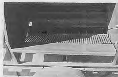
Fig. 4 Pod conveying unit. A) Auger conveyor, B) Sliding tray.
