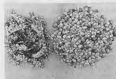
Fig. 6 Threshed fruitlets produced by an experimental drum thresher.
