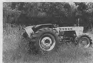
Fig. 2 Illustration of lack of appropriate back-up service and lack of standardization in manufacture. The tractor on the foreground became redundant from lack of spares. Poor workmanship on mass produced punch-planters on the back ground led to rejection by the intended users. Such may be avoided by user survey and standardization in manufacture processes and for quality control.
