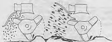
Fig. 6.2 Side views of rotary tiller.
