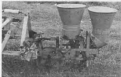
Fig. 4 Planter prototype during test on a field with grass.
