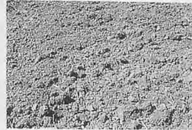
Fig. 15 Rotary tilled plot at speed-II and rear shield down.
