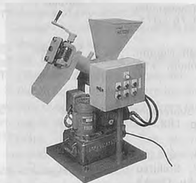
WORLD Squeezer LP-5. The world's first continuous rice-bran vegetable seeds oil extraction equipment (SQUEEZERS). Type: LP-5 (ring system), Capacity: 8kg/h (Rice bran 5), Residual oil: 15% (Rice bran 10%), Power required: 0.4kW, Net weight: 90kg, Cylinder pressure: 5ton, Size in m: 1W x 0.5L x 1.2H.
