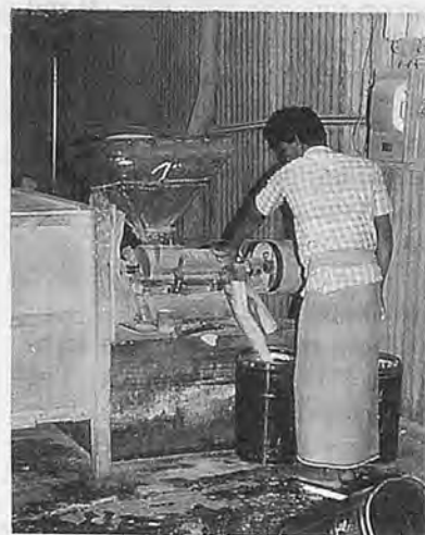
Fig. 2 Milling operation of paddy in Engleberg huller.
