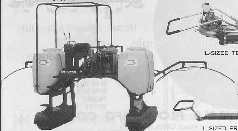
OMS-2 Riding type pest control machine
