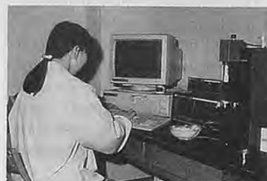
Fig. 4 Texture valuation test for boiled rice.
