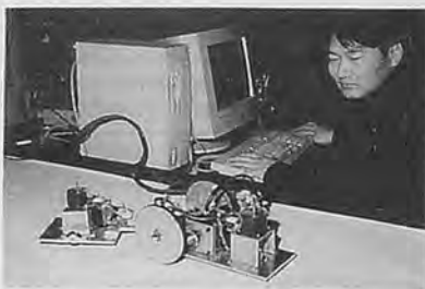
Fig. 3 Computer control of motion of a tractor-trailer combination model.
