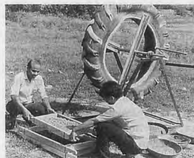
Fig. 3 Tyre type seed pelleting machine.
