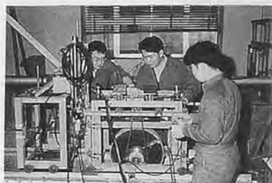
Fig. 2 Experimental apparatus for a travel performance test of a wheel.
