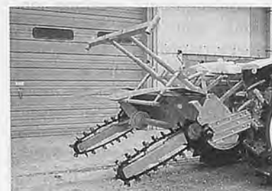
Fig. 4 Newly developed trenching drainer.
