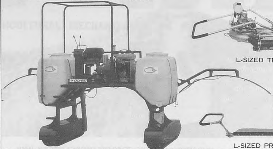
OMS-2 Riding type pest control machine
