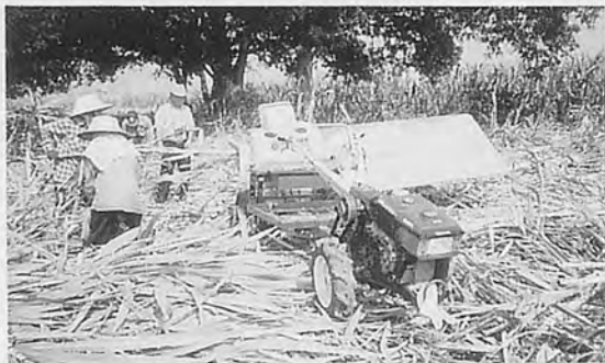
THE BABY LEAF STRIPPING MACHINE (MBC-250C)
