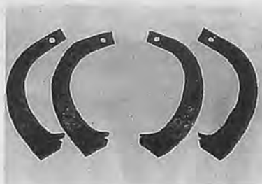
Fig. 6 Commercially available low-cost power tiller tynes manufactured from old leaf springs of trucks.
