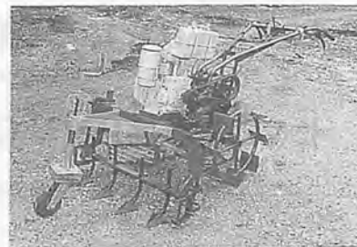
Fig. 1 Self-propelled onion digger windrower showing different functional units.
