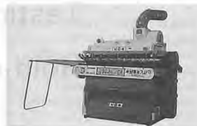
Fig. 1 Hold-on paddy thresher (imported version).
