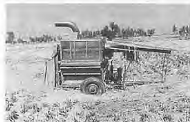
Fig. 2 Hold-on paddy thresher (FMI-modified version) shows the new base structure, tray modification, power transmission changes, addition of transport wheels and toeing hitches.
