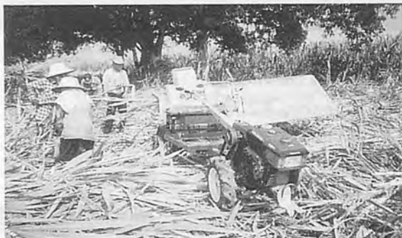
THE BABY LEAF STRIPPING MACHINE (MBC-250C)
