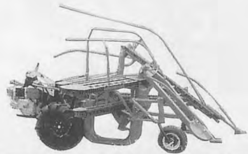
THE SMALL WALKING TYPE HARVESTER (NB-11)
