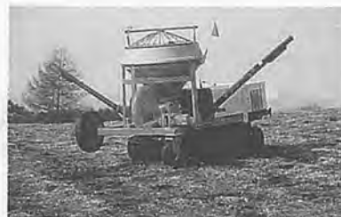
Fig. 6 Radio control fertilizer spreading machine designed for use on sloping terrain. We can avoid dangerous work, or operating a fertilizer spreading machine on sloping grassland owing to this radio control machine.
