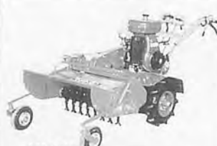
MH-750 HAMMER KNIFE MOWER
