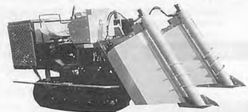
THE RIDING TYPE HARVESTER (TK-5...60PS)
