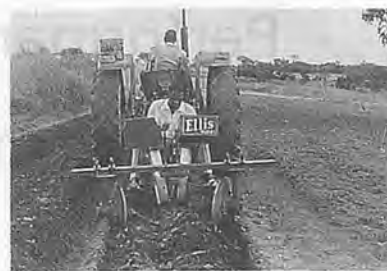
Fig. 2 Tractor mounted imported semi-automatic transplanter modified at national centre for agricultural mechanization, Nigeria, to plant cassava setts in operation.
