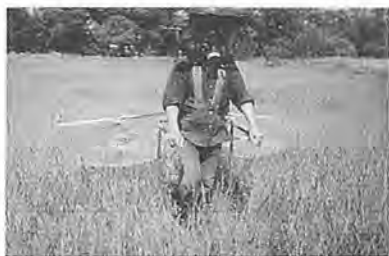
Fig. 4 Knapsack electrostatic sprayer with plastic shields.
