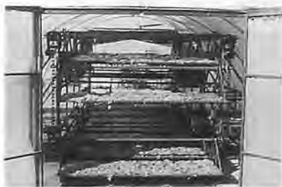
Fig. 2 Rotating trays within solar tunnel drier.
