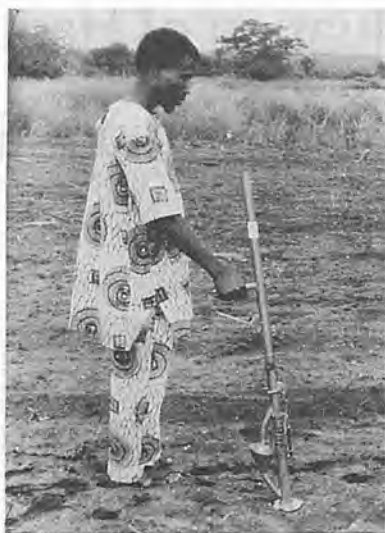
Fig. 2 AIT fully-automatic manually-operated Jab planter in operation (Planter II).
