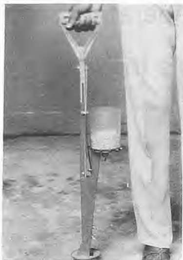
Fig. 1 Italian fully-automatic manually-operated Jab planter in operation (Planter I).
