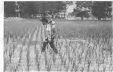
Fig. 2 Sprayer converted into pull-along type.
