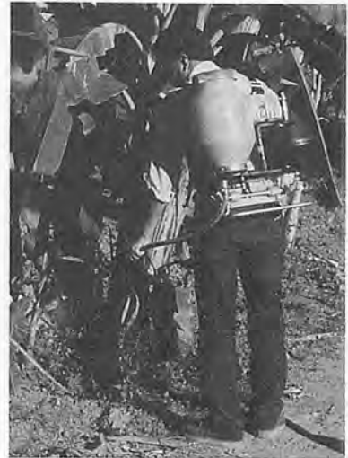
Fig. Safety and quickly Swissmex-152 granule applicator places precise dosage of fungicide or nematicide at base of tree.
