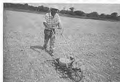
Fig. 3 Field operation of manually-operated electrostatic planter.
