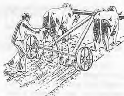
Fig. 7 Intercultivation machine with Stage II rigid transport wheels, tool depth adjustment and lift, and operator's seat.
