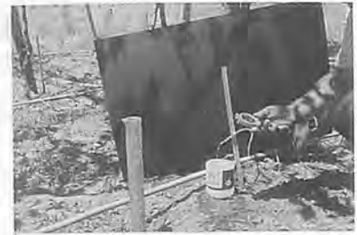
Fig. 3 Calibrating a low-cost polytube emitter in the field.
