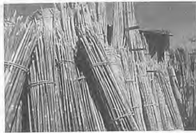
Fig. 1 Locally available bamboos used for drip pipeline.
