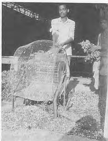
Fig. 3 Power-operated single drum groundnut thresher.
