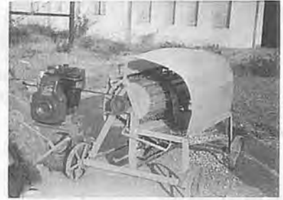
Fig. 2b Power-operated double drum groundnut thresher (driven by power tiller).
