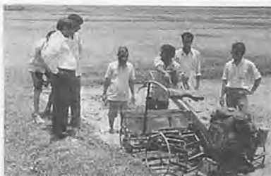
Fig. 3 Operation of the pre-germinated paddy seeder.
