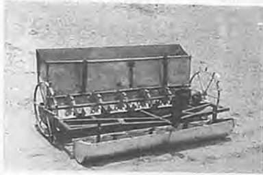
Fig. 2 Power tiller-operated pre-germinated paddy seeder.
