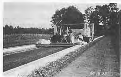
Fig. 2 Single tire tester in conjunction with soil-bin dynamometer car.
