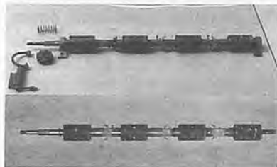
Fig. 3 Seed metering roller and fertilizer agitator assembly for paddy seed (top) and for soybean and maize (bottom).
