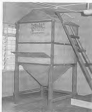
Fig. 9 The wooden multi-produce silo, designed and fabricated at the Federal University of Technology, Akure, Nigeria.
