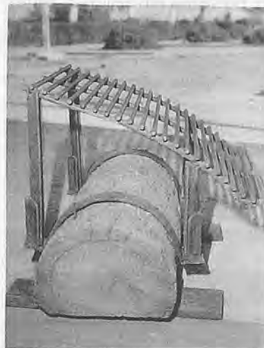
Fig. 1 Threshing aid for manual paddy threshing. ① 12 mm diam mild steel rod 560 mm long, 3 nos.; ② 10 mm diam mild steel rod 400 mm long, 20 nos.; ③ 33 × 33 mm angle legs, 210 mm high front legs, 2 nos., 330 mm high rear legs, 2 nos.; ④ 50 × 6 mm mild steel flat, 400 mm long, bent to curve, 2 nos.; ⑤ 300 mm diam coconut trunk 750 mm long, 1 no.; ⑥ 100 × 15 mm wooden plank, 500 mm long, 2 nos.
