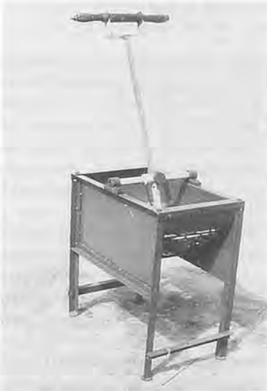
Fig. 5 Modified manual groundnut decorticator Model-II with 9 × 45 mm slotted sieve.
