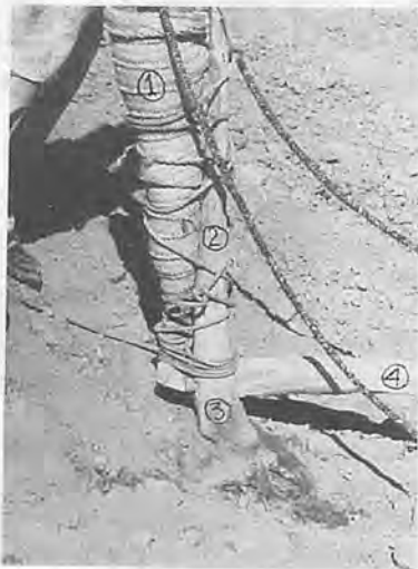
Fig. 1 Seed distribution system and shape of local drill: ① Seed metering system; ② Handle; ③ Share; ④ Beam connects with camel.
