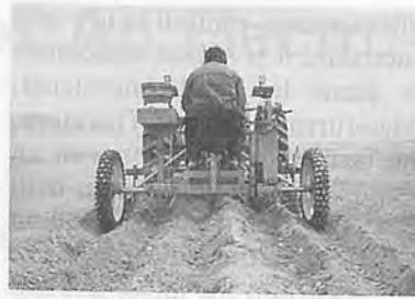
Fig. 4 Field performance of the seed drill showing the placement of seeds and the construction of the ridge-furrow system.
