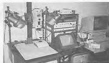
Fig. 2 Video analyzer system for motion analysis.
