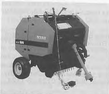
STAR Mini-Roll Baler MRB 0810. Automatic pick-up, rolling and ejection. One bale every 30 seconds. Handy bale size (50cm in diameter and 70cm long). Required tractor horsepower: 18-30 HP.
