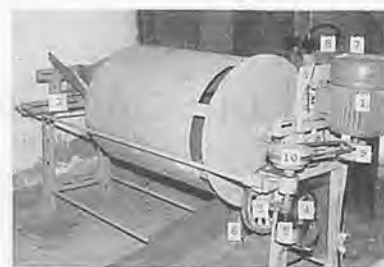
Fig. 1 Grain dryer. ① Electric motor; ② Iron stand; ③ Spur gear; ④ Worm wheel; ⑤ Worm; ⑥ Sieve; ⑦ Gas meter; ⑧ Sand heating pan; ⑨, ⑩ Step pulleys.
