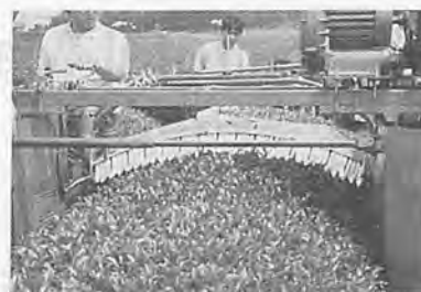
Fig. 3 Field test of tea-leaf plucking machine.
