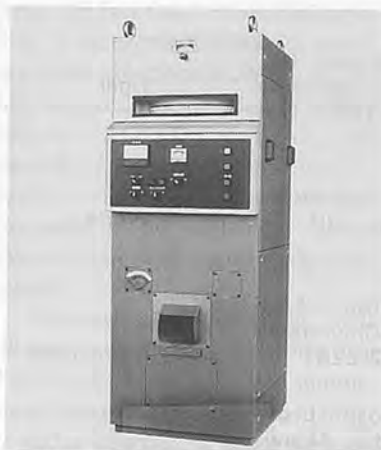
YAMAMOTO Rice Whitening Machine VP-2201F. Keeps original shape and flavor of rice by high performance of moving screen mechanism and natural flow-down system. Capacity: 1.0-1.8t/hour. Power required: 22kW and 0.23 kW.
