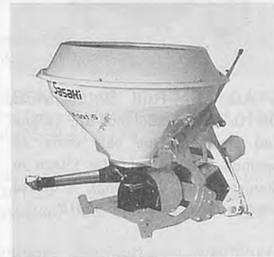
SASAKI Fertilizer Spreader BF-300. The lever type action controls the amount of application with high accuracy. Application width: 10-12m. Hopper capacity: 300ℓ. Required tractor horsepower: 20-50PS.
