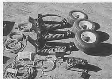
Fig. 1 Major components of the Microtek Automatic Depth Control System.
