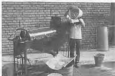
Fig. 6 Vegetable seed extracting machine being used for tomato seed extraction.
