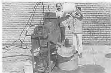
Fig. 5 Vegetable seed extracting machine being used for chillies seed extraction.
