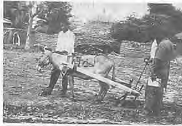
Fig. 3 Field testing of the donkey-drawn cultivator.
