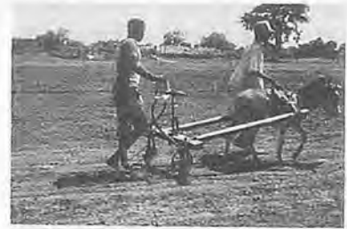
Fig. 4 Field testing of the donkey-drawn two-row hill-seeder.
