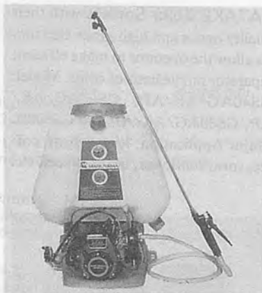
MARUYAMA Portable Power Sprayers MSO55D. Engine: Air-cooled, 2-cycle, output 22.6cc, Pump: Suction capacity 5.1l/mm, max pressure 25kg/cm 2 , Weight: 8.5kg.
