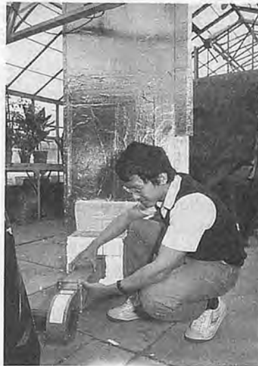
Fig. 5 Side view of store showing fan inlet.
