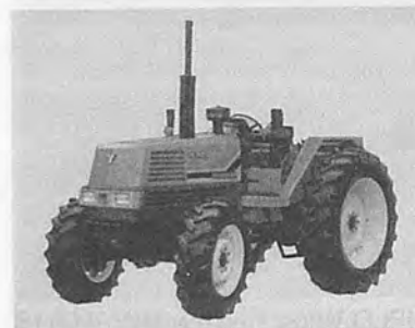
YANMAR Diesel Tractor F97. Engine: vertical, 4-cycle, water-cooled diesel 97HP/2,200rpm. Weight:
