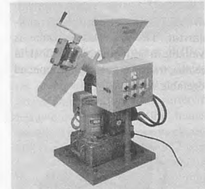
WORLD Squeezer LP-5. The world's first continuous rice-bran vegetable seeds oil extraction equipment (SQUEEZERS). Type: LP-5 (ring system), Capacity: 8kg/h (Rice bran 5), Residual oil: 15% (Rice bran 10%), Power required: 0.4kW, Net weight: 90kg, Cylinder pressure: 5ton, Size in m: 1W x 0.5L x 1.2H. ■■
