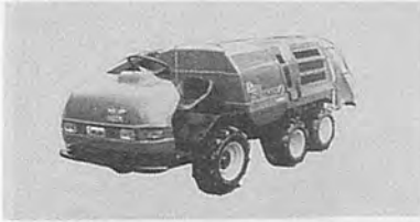
SASAKI Speed Sprayer RS-660Z. Engine: water-cooled diesel 32HP. Drive system: 6-wheel drive. 600ℓ tank. Air output: 560m 3 /min. Pump output: 94ℓ/min. Dry weight: 1,220kg.
