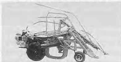
THE SMALL WALKING TYPE HARVESTER (NB-11)
