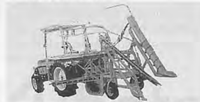
THE RIDING TYPE HARVESTER (NB-15T)
