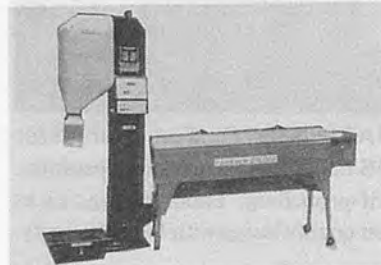
TIGER KAWASHIMA Rice Combi and Grader. Rice grading machine and automatic weighting and packaging.
