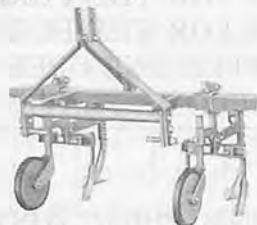
Double-Row Cultivator TBC (Tool Bar & Cultivator)
