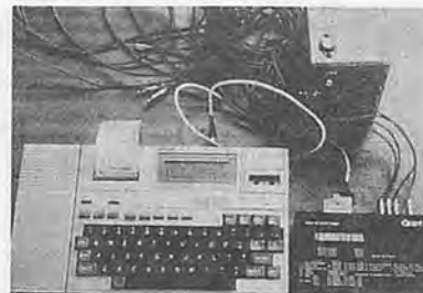
Fig. 2 The power supply box, data logger and the portable computer.
