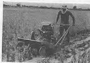
Fig. 3 Hydro tiller in operation under normal field conditions.
