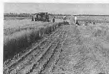
Fig. 4 The stubble and the windrow of the stripped rice straw (right) after the WTC mounted with reaper.
