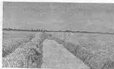
Fig. 12 Laying out polythene sheet to determine conveying loss.
