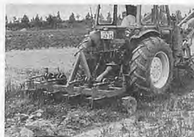
Fig. 1 Developed 4-shank type vibrating subsoiler—Each shanks were oscillated by PTO shaft in optimal arrangement. Amplitude and frequency were set at 50mm and 3 Hz. As the draft was reduced to the 50%, a medium size tractor was able to do the subsoiling practice at a high efficiency.
