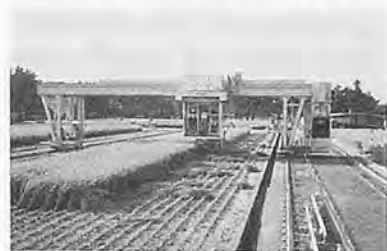
Fig. 2 Crop cultivation systems with a gantry.
