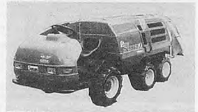
SASAKI Speed Sprayer RS-660Z. Engine: water-cooled diesel 32HP. Drive system: 6-wheel drive, 600l tank. Air output: 560m 3 /min. Pump output: 94l/min. Dry weight: 1,220kg.
