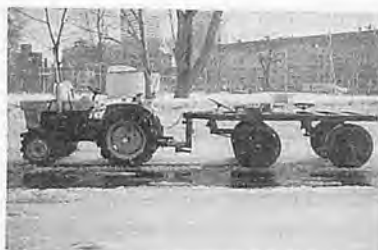
Fig. 2 Combination of tractor and trailer—This trailer was developed for investigating the stability of a tractor-trailer combination. The trailer was equipped with a steering system and it was controlled by a computer.
