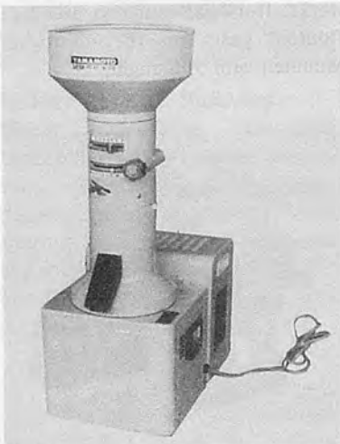
YAMAMOTO Test Whitening Machine VP-30T: Type of milling: vertical. Weight: 24kg. Power required: 0.3kW. Capacity: 30kg/h. Hopper holding capacity: 5kg.
