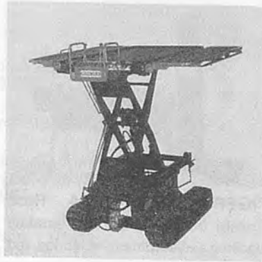
NOZAWA Fruits Worker. Mobile elevating platform for orchard works: from harvesting to pruning. Control gears on the platform. Mounted with 5PS engine.
