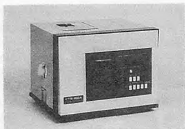
SHIZUOKA Single Grain Moisture Meter CTR-160A. For larger size grains (maize or soybean). Measures a lot of 20 grains.
