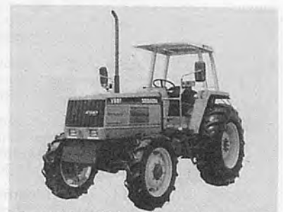
SHIBAURA Tractor Stiger V. Eased works with car-ride feeling. Synchromesh transmission and column shift employed. Engine horsepower: 70-80.
