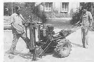
Fig. 2 Controlling the depth by hand-wheel.
