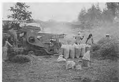
Fig. 6 Modified dual-mode all-crop thresher being used by farmers for threshing paddy in the Nile Delta. AK 1989.
