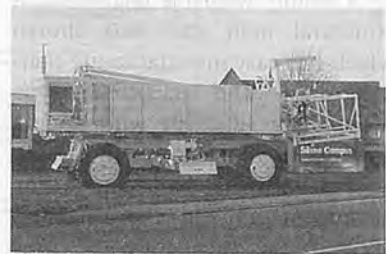
Fig. 1 Date palm service machine in transport position.
