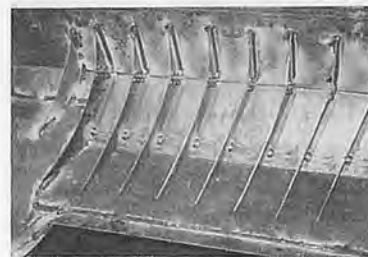
Fig. 4 Adjustable angle louvers in the threshing drum cover of the modified dual-mode all-crop thresher. Louvers are shown in the axial-flow mode for threshing paddy.
