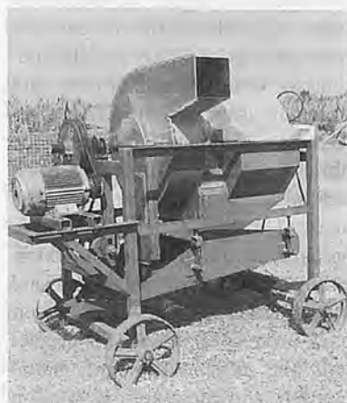
Fig. 7 A soybean thresher developed with the collaboration of a local manufacturer.
