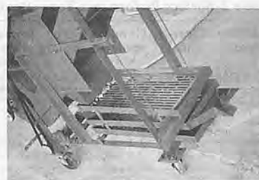
Fig. 10 G.I. sheet screens with slot along the direction of oscillation.
