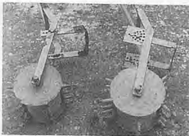
Fig. 6A Product development of a manual weeder to facilitate fabrication (Left: Frame fabricated from 40 x 4 flat with V-shaped cutting blade, Right: Multiple hole frame fabricated from 4 mm sheet with crescent-shaped blade).
