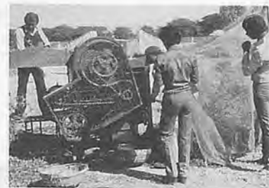
Fig. 6B Product development of a semi-axial flow multi-crop thresher with spiral aspirator blower.
