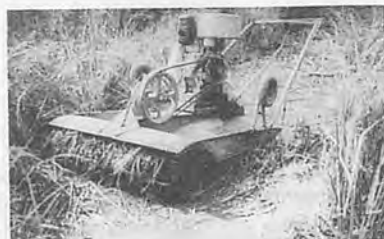
Fig. 4 Weeds and stubble clogging original rotor.
