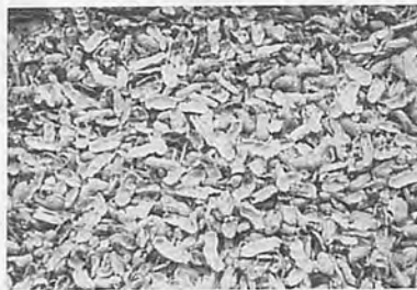
Fig. 13 Shells blown with radial bar type concave.
