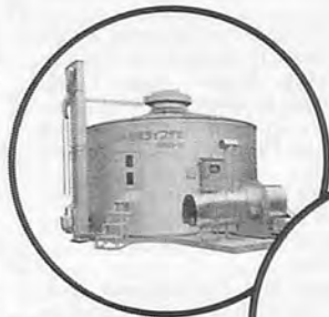
DRYING & STORAGE BIN
