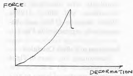
Fig. 3 Force-deformation curve of yam tuber
