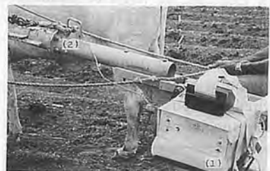
Fig. 2 Data acquisition system with printer. 1—System, 2—Pull force transducer.
