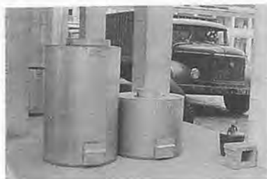
Fig. 5 Metal bins. Capacity: 200 and 400 kg.
