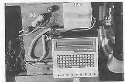
Fig. 5 Data acquisition system components. 1—Data acquisition system, 2—Battery, 3—Pull force transducer.
