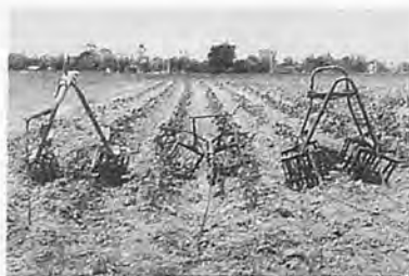
Fig. 7 Prototype rotary weeders: left to right - Strad, Emcot-attached (interrow) rotary weeder, High-clearance straddle-row rotary weeder.
