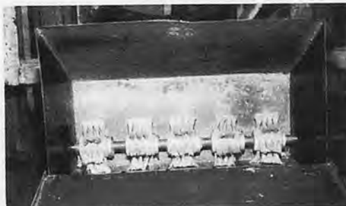
Fig. 6 Nylon brush for seed metering.
