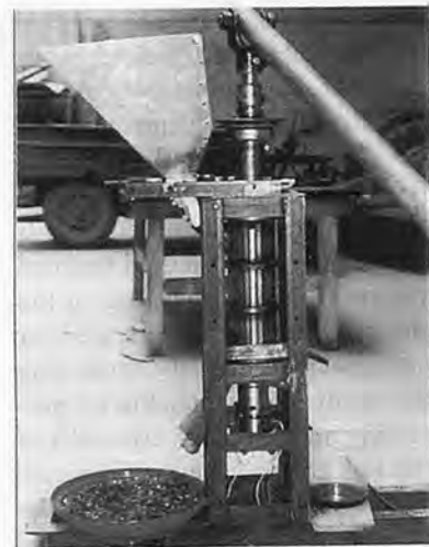
Fig. 3 Designed and fabricated multi-drive screw expeller under test.
