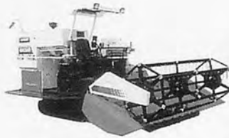
Full Rubber Crawler, 76hp 2.06m harvesting width
