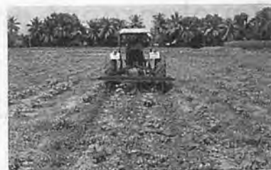
Fig.1 Tractor drawn weeding cum earthing up implement.
