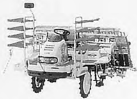
Water-cooled Diesel mounted, 8rows
