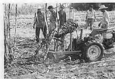
Fig. 11 A walk-type mini-harvester developed in CSRDC in 1994.
