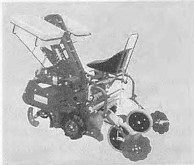
SUKIGARA ABLE Potato Planter TAP-100MT. Planting, ridging, ground cover laying in one operation.
