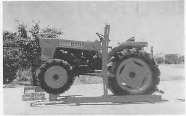
Fig. 7 The device in action-view from the side. The tractor in its raised position resulting in an angle between the fixed and moving vertical tubes.
