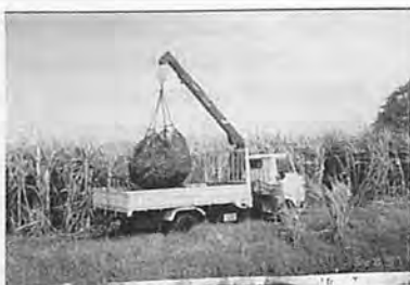
Fig. 7 A special purpose lifter is used to lift and load, which is bag dumped from TS2001.
