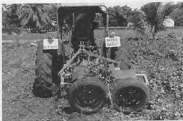
Fig. 2 Operational profile of cotton stalk puller.
