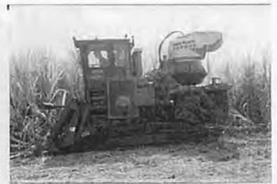
Fig. 6 A specially modified model of chopper harvester for the Thai sugar industry, TS2001, in action.
