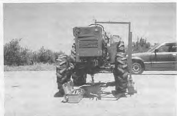
Fig. 5 Photograph showing the strain indicator connected to the load cell.
