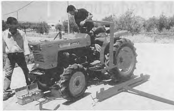
Fig. 6 Tractor operators tightening the moving vertical tube on the tractor by lowering the power screw to encounter the first surface from the top of the tractor.
