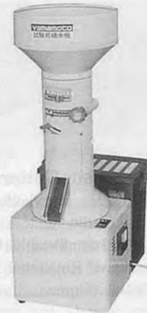
YAMAMOTO Rice Whitener Ricepal Series Model VP31T. High recovery rate. Immatured rice can be milled. No remaining rice in the machine. Easy-to-change milling screen. Durable construction. Milling system: vertical type single pass, Size (H x W x L):850 x 330 x 450mm, Weight: 24kg, Power required: 0.3kW, Electric mains: single phase 100V (50/60Hz), Capacity: 30kg/h, Rpm:1440/1730, Hopper holding ca-
