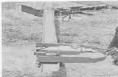
Fig. 2 Dynamometer attachment for draught measurement.
