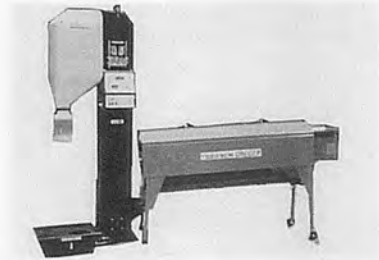
TIGER KAWASHIMA Rice Combi and Grader. Rice grading machine and automatic weighting and packing.
