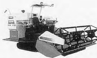
Full Rubber Crawler, 76hp 2.06m harvesting width
