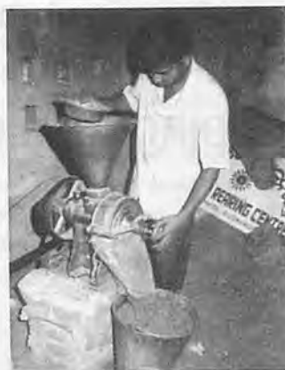
Fig. 10 Milling of turmeric in local flour mill.
