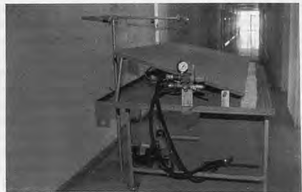
Fig. 2 Side view of nozzle spray distribution test stand showing nozzle holder and pressure regulator.
