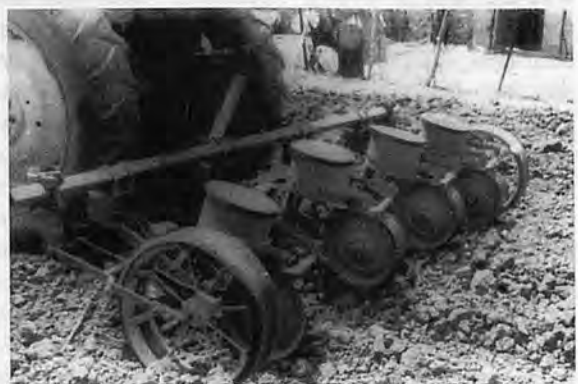
Fig. 1 The shape of the improved crop planter with attached assembled furrow wheels.
