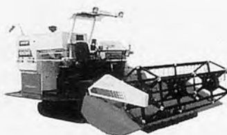
Full Rubber Crawler, 76hp 2.06m harvesting width
