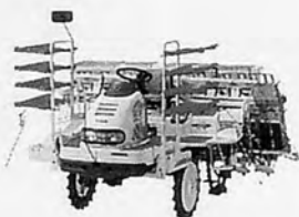
Water-cooled Diesel mounted, 8rows
