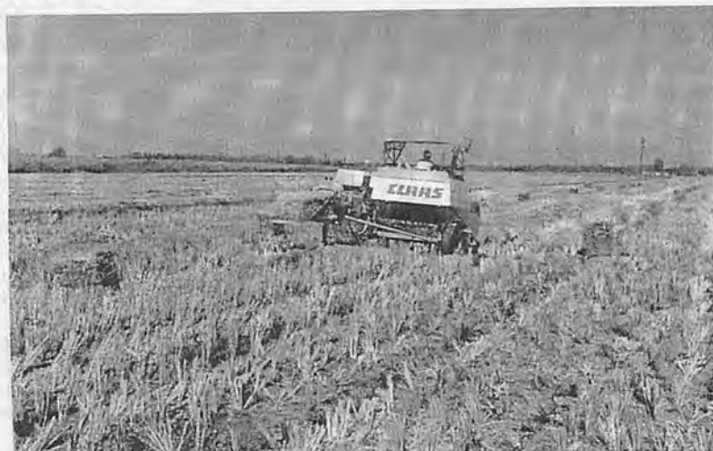
Fig. 1 A view of conventional field baler during baling of combine harvested paddy straw.
