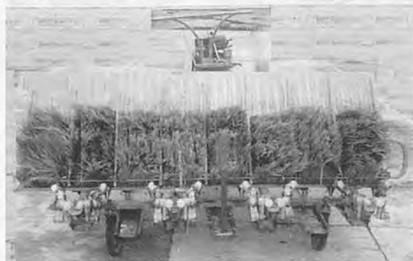
Fig. 3 Self-propelled rice transplanter used in the experiment (rear view).
