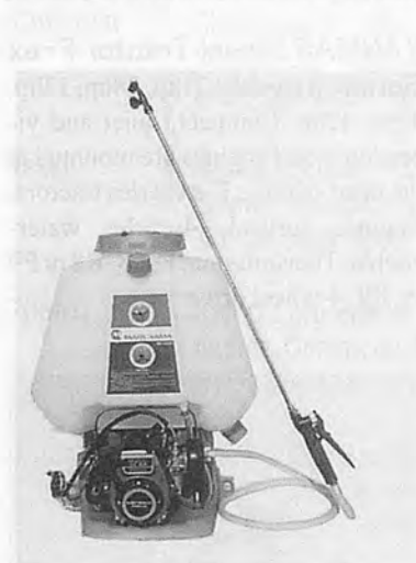
MARUYAMA Portable Power Sprayers MSO55D. Engine: Air-cooled, 2-cycle, output 22.6cc, Pump: Suction capacity 5.1/mm, max pressure 25 kg/cm 2 , Weight: 8.5 kg.
