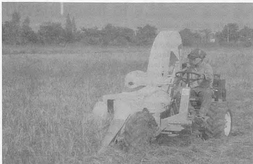
Fig. 5 Cirad stripper, Rth model with winnowing device in Thailand.
