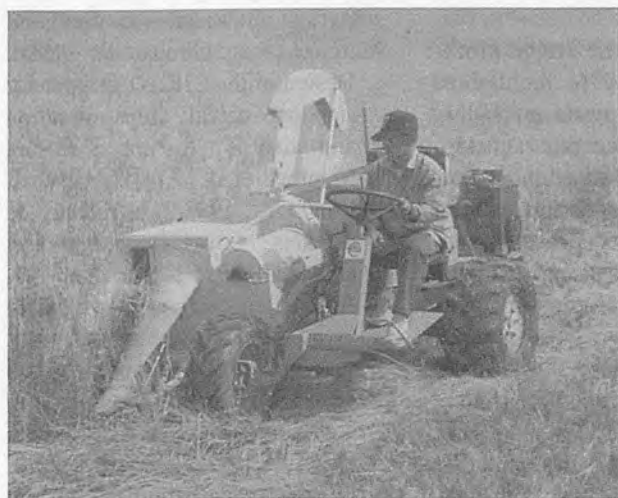
Fig. 6a Cirad stripper, Rth model without winnowing device in Thailand (front view).
