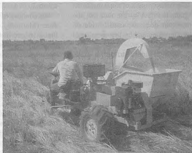
Fig. 6b Cirad stripper, Rth model without winnowing device in Thailand (back view).
