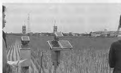
Fig. 4 Water management system for paddy field attached with auto irrigation gate wireless data communication device and solar batteries.
