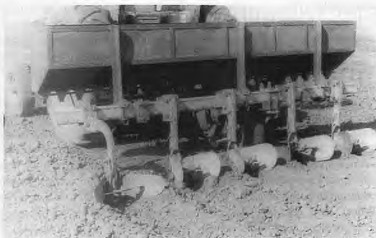
Fig.2 The fabricated combined operations machine for wheat crop sowing in working.
