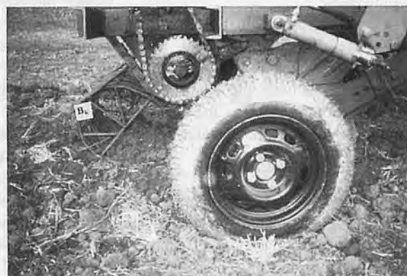
Fig. 9 Side view of cassava root lifter/elevator when lowered into harvesting operation position.
