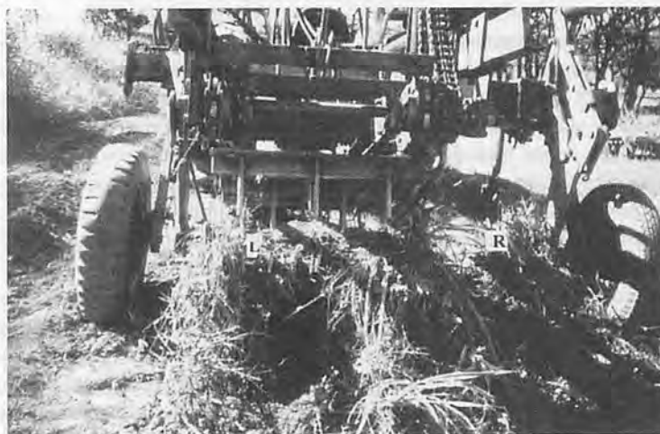
Fig. 9 A photograph showing the rear view of the implement with the harvesting aid fully in the cassava harvesting position and illustrating the differences between the left (L) and right (R) rows.
