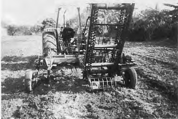
Fig. 10 A photograph showing the rear view of the lifter/elevator, with the bucket, B k , about to comb through the soil.
