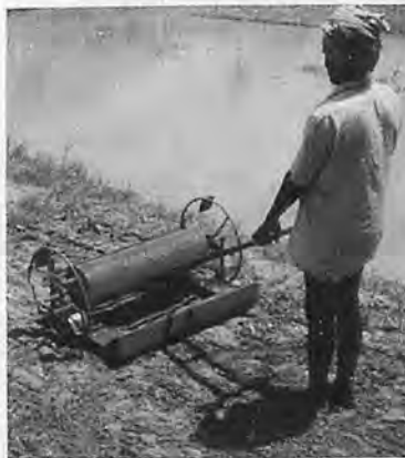
Fig. 2 5-row drum seeder of CRRRI (manually pull type).
