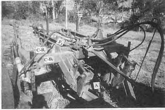
Fig. 13 A photograph of the modified frame of the Ikeda harvesting aid, showing the rear cross-beam, C-B 2 , moved closer to the front cross-beam, C-B 1 , and the frame of the conveyor rake, F 2 moved forward closer to the blades of the harvesting aid, A.
