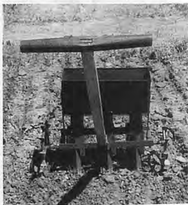
Fig. 1 3-row manually pulled CRRRI seed drill.
