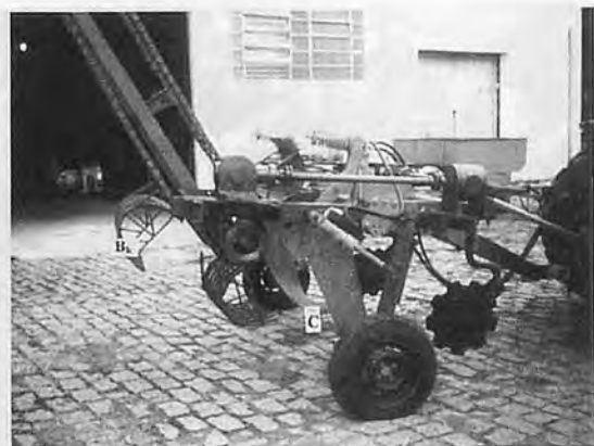
Fig. 7 The cassava root lifter/elevator raised into transport position outside the workshop. C - harvesting aid; B_k - elevator bucket.
