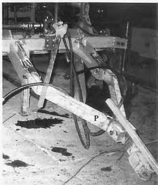
Fig. 4 Photograph showing the constructed pull-bar, P, welded to the original lower-link hitching members of the Ikeda harvesting aid.
