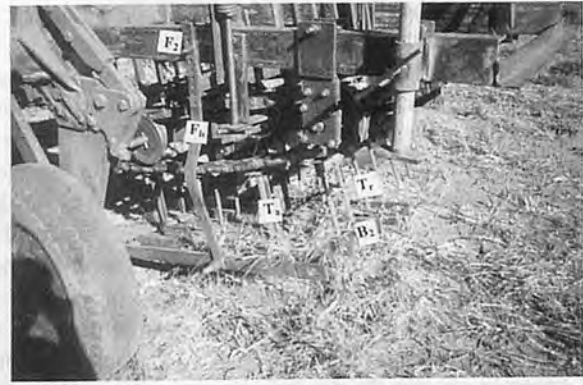
Fig. 14 A photograph of elongated tines, showing rows of round rod tines, T 1 , alternating with rows of angle-iron tines, T 2 , spaced 45mm apart and reaching to 25mm above the platform formed by the extension bars, B 2 , hung with a pair of bars, F b , from the frame, F 2 , of the conveyor rake.
