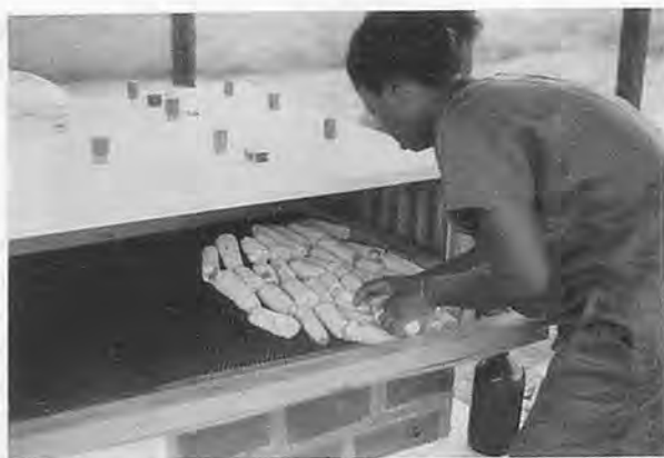
Fig. 3 An operatress setting wet maize on-cob for drying in the universal dryer.
