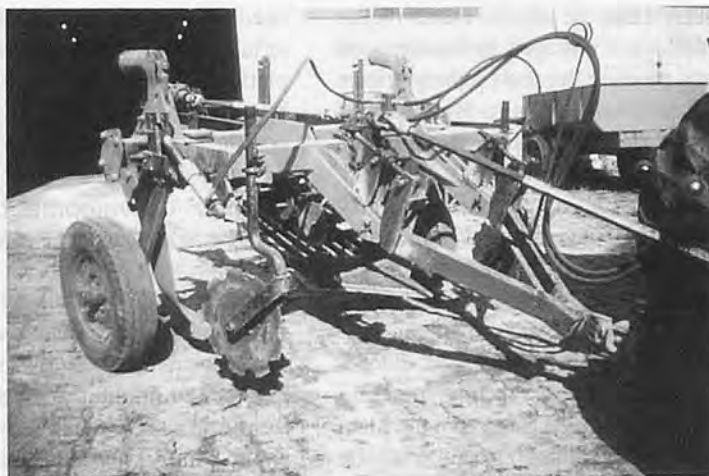
Fig. 5 Photograph of implement raised into transport position.
