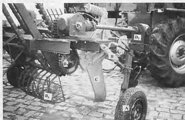
A - transport/guage wheels; B - hydraulic ram; C - right-side shank/blade of harvesting aid; D_1 - 2:1 gear box; D_2 - 2 nd gear box; D_3 - 3 rd gear box; D_4 - bottom/driving sprocket of the chain-and-sprocket elevator system. B_k - elevator bucket.
