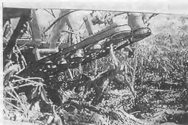
Fig. 5 Vee-belt cassava uprooter/lifter prototype from Interplan Company in Itarere, S.P., Brazil.
