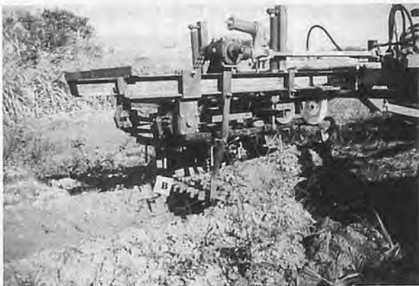
Fig. 7 A photograph showing the extension bars, B, being lowered into working position.
