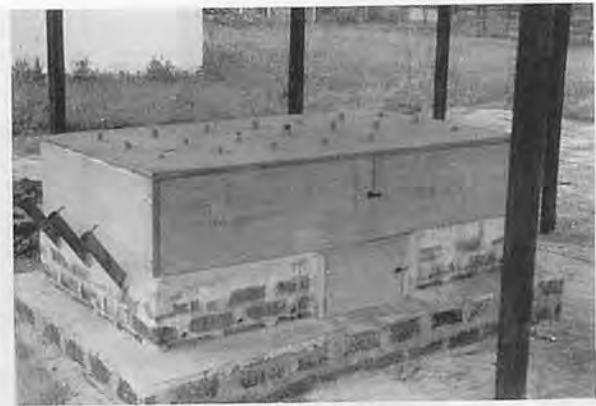
Fig. 2b The universal dryer. Note the three left exhaust pipes from the heating chamber. The air pot is enclosed.
