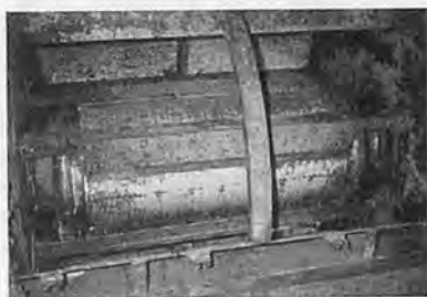
Fig. 2 The inner scraper for cleaning of mucilage.
