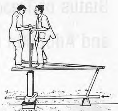
Fig. 5 Pump operation by two adults.
