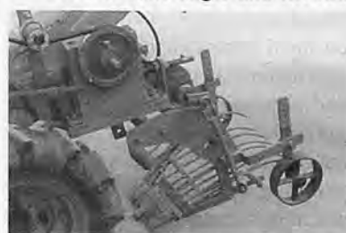
Fig. 1 Power tiller-operated turmeric harvester.
