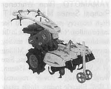
MAMETORA Power Cultivator SRV4F. Wide range use: cultivation to riding, Mounted with 7 PS engine.
