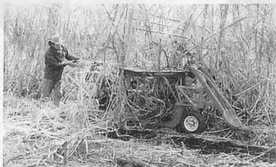
THE SMALL WALKING TYPE HARVESTER OPERATION SCENE
