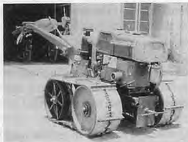
Fig. 2 Power tiller fitted with rubber track.
