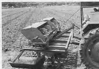
Fig. 2 Broad bed former cum-seeder attachment to tractor-drawn cultivator.
