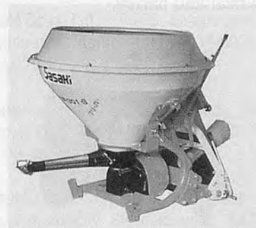
SASAKI Fertilizer Spreader BF-300. The lever type action controls the amount of application with high accuracy. Application width: 10-12m. Hopper capacity: 300l. Required tractor horsepower: 20-50PS.
