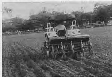
Fig. 1 Basin lister cum-seeder attachment to tractor-drawn cultivator.
