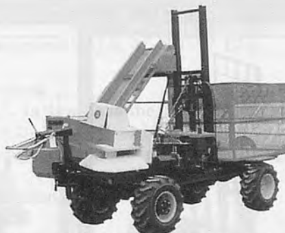
THE SMALL LEAF STRIPPING MACHINE (KC-2 MODEL)
