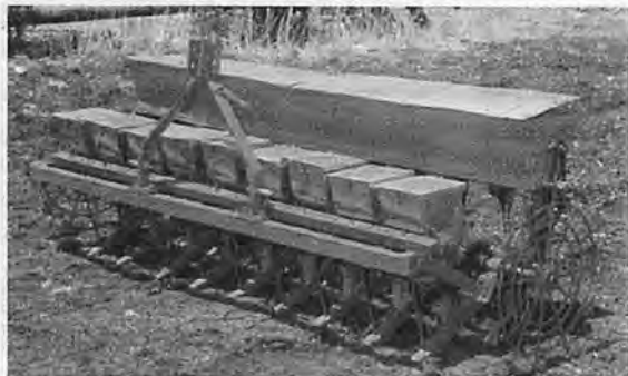
Fig. 1 Tractor-drawn multi-crop planter.
