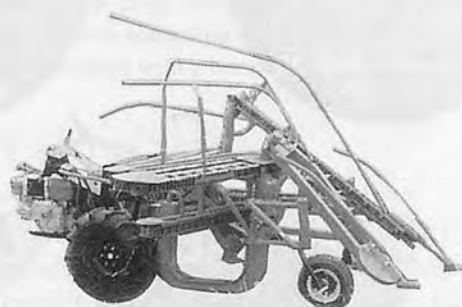
THE SMALL WALKING TYPE HARVESTER (NB-11)
