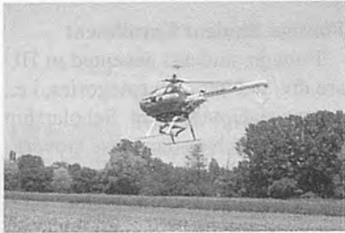
Fig. 1 Unmanned helicopter for precision agriculture.
