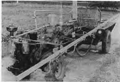
Fig. 1 Mounting of sprayer system on carrier.
