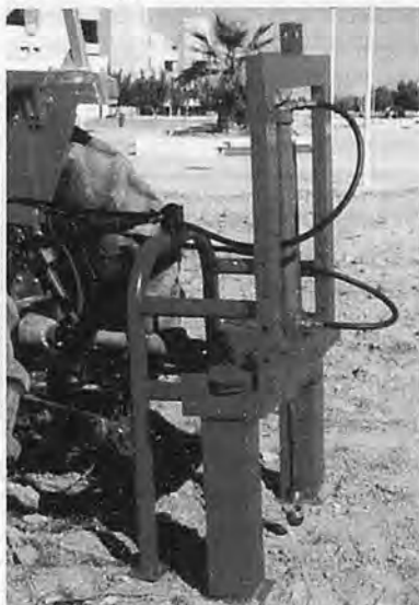
Fig. 1 The hydraulically-powered soil core sampler mounted on a tractor.
