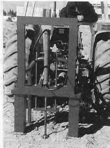
Fig. 8 The HPSCS shown hitched behind the tractor ready to probe soil sampler.
